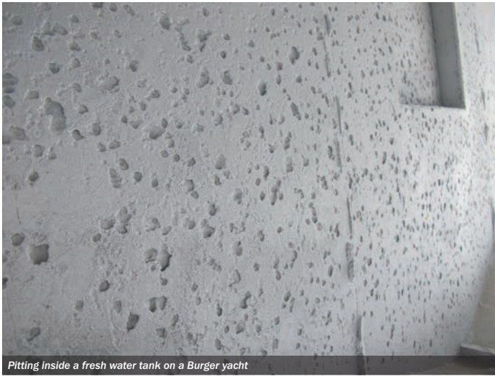
Pitting inside a fresh water tank on a Burger yacht
